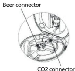
3. Open the beer dispenser and place the well assembled keg in the cooling cavity. Connect the CO2 connector hose and the beer drain hose to the keg lifter hose connector.
