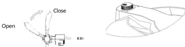
Loosen the sheath of the CO2 bottle (as shown in Figure A), insert a 16g CO2 cartridge into the sheath (Figure B), and screw the tight sheath until you hear a "click" (Figure C), which indicates that the cartridge seal has been pierced and that the CO2 gas can flow freely into the drum. Make sure that the cylinder sheath is firmly fixed in order to prevent CO2 from escaping. After that, put the sheath of the CO2 bottle in the top cover.
